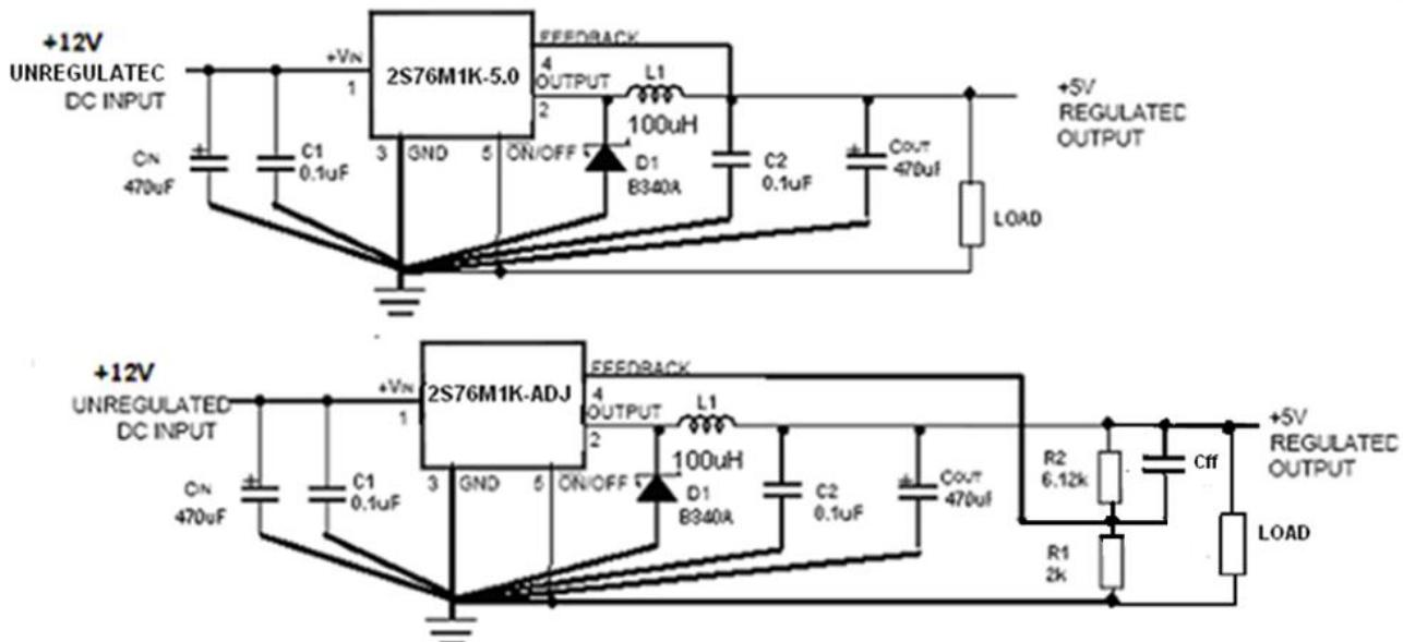
$$V_{OUT} = V_{REF}(1 + \frac{R_2}{R_1})$$
