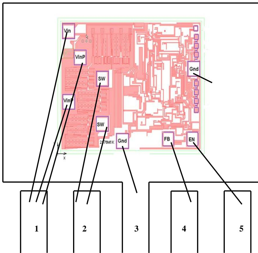
The wire diameter is 50µm
