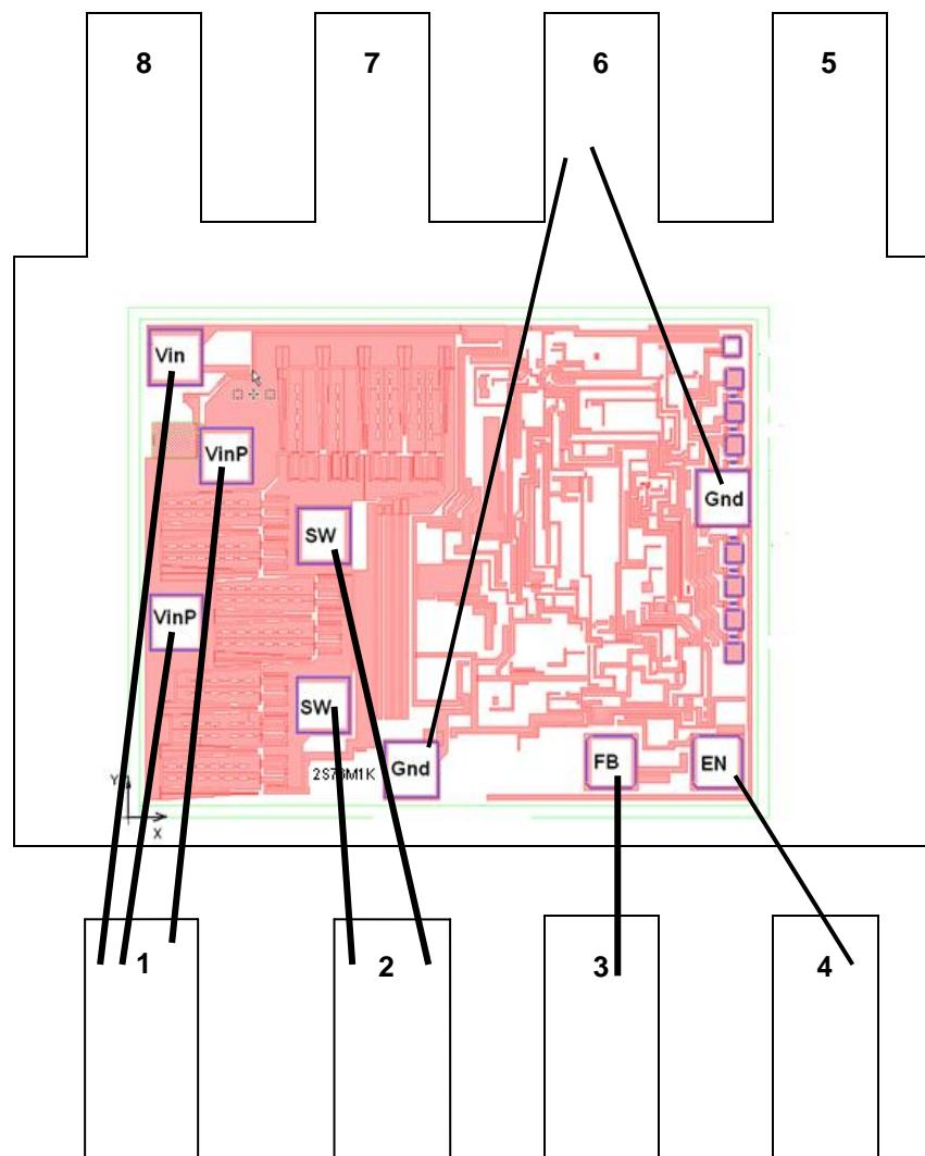
The wire diameter is 50µm
