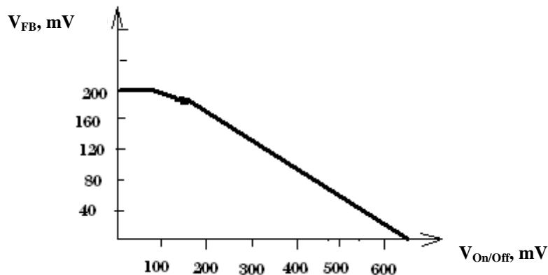
Fig.1. Dimming voltage (typical),  $V_{FB} = f(V_{On/Off})$
