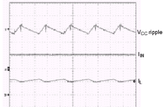
Figure 7. Boost Input Voltage and Current Ripple Waveforms
