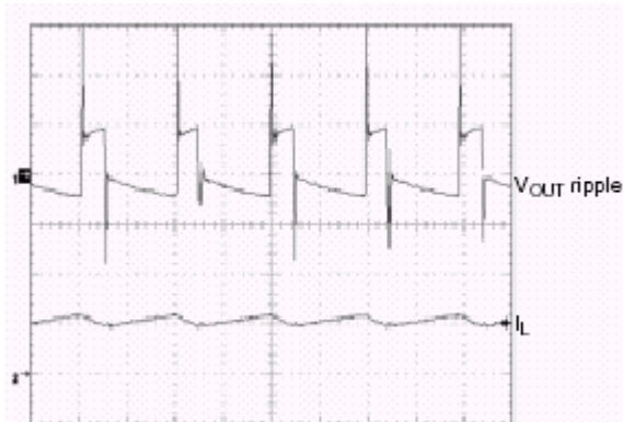
Figure 9. Typical Output Voltage Ripple
