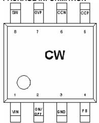
SOP-8 with Exposed PAD connection to Gnd on the bottom of Package
