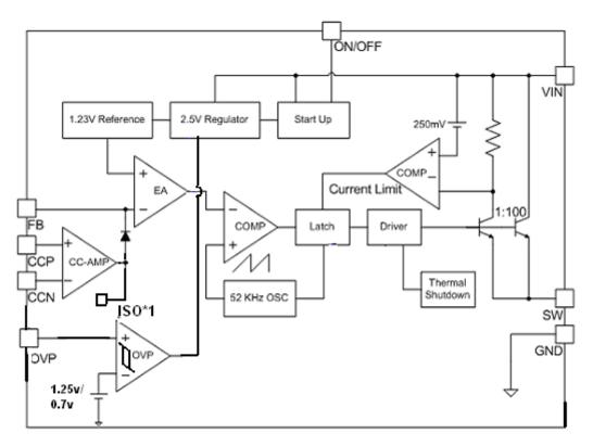
Note \*1: There is the reserved PAD ISO at output of Op Amplifier. It allows leave ISO open [Version 1] either connect ISO to the pin FB (shorting the diode) [Version 2] during packaging.
