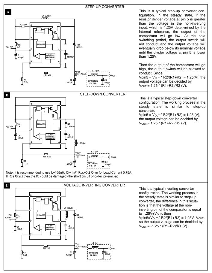
Inv № 53334063CM3K1.2A STEP-DOWN / STEP-UP / INVERTING DC-DC CONVERTER
